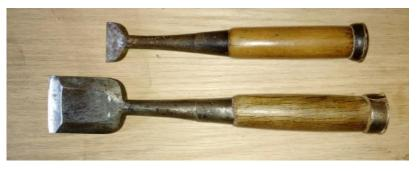
At the top is what used to be an excellent chisel, but is now just, to be polite, a nub; the lower one is a still usable example for comparison. Why was this chisel still in the tool roll? It's too short to sharpen. It's too short for self-defense. In a stretch, one might use it as a scraper but there were six of them. Conclusion: the old carpenter couldn't bear to throw it out. Worse: why do *I* still have the nub? Conclusion #2: I need a twelve step program for tool addicts.
