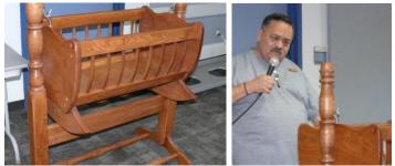
Rocking the cradle **Fred Sandoval** explained how he carefully mortised and aligned the joints to accommodate the slats for the side of the cradle. The cradle is of red oak which Fred found hard to turn unless you have sharp tools. Fred finished with Hydrocoat.
