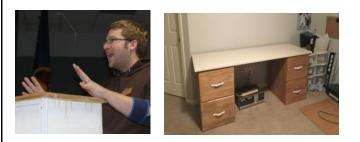
A fun first time project for **Mark Womack** was a desk that his wife pretended to like to two years. So Mark came up with a new design using Sketchup. Joinery is pocket holes and glue. Handles from Hobby Lobby. Mark finished with water borne polyurethane because oil based yellows over time which Mark didn't want.
