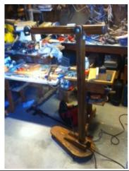
This is an adjustable boom shop light I made a few years ago. The reason I am showing again is that I put casters on it and it is much easier to move around when I need additional light in an area. Easy to make, light is from an old tract lighting system that I recycled.—**Mike Turner**
