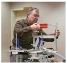
After retiring from his process engineering job, Inventor Matthias Wandell developed a working mortise and tenon machine using the principle of thepantograph to reduce a large scale template to a smaller size de-
