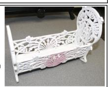
Baby Cradle pattern was on a scroll saw web site, and was cut out on 1/4" plywood with 2/0 spiral blade and painted with spray paint. — Rick Spacek
