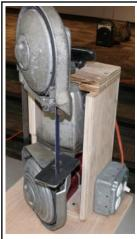
Metal cutting portable bandsaw (Milwaukee portalign band saw) mounted in a cabinet in the vertical position to cut small pieces of metal. It is designed to mount on your workbench with a clamp to secure it or you can remove the tool and use it. There is an electrical switch with a receptacle mounted on
