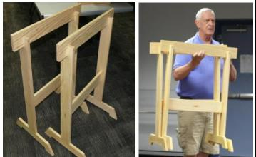
From three eight foot one by fours, **Jack Baile** made two Kernov style sawhorses of pine. The top cross pieces are not glued but doweled to facilitate replacing for repair. Download plans for Jack's saw horses (PDF file) from the WWCH website. Thanks, Jack.
