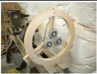
David Janowitz-Here's a steady rest I built from Wink-wood plywood, a few nuts and bolts, and some 3" urethane ball-bearing wheels. This should work great for medium to large spindle
