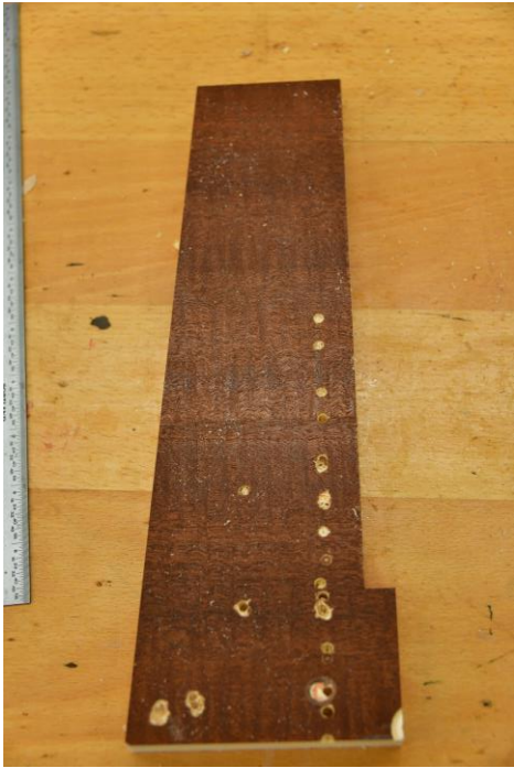
A simple taper jig, made from a well-used piece of scrap
