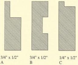
A is 3/4" x 1/2" and is used for rabbeting side pieces to allow top and bottom panels to be inset. This is used if the top/bottom joints are not seen, as in kitchen cabinets or furniture with separate tops. The 1/2" ledge allows plenty of room for a fastener.
