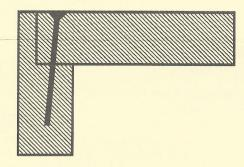
B is 3/4" x 1/4" and is used for fixed shelves or dividers. The 1/4" bearing is plenty. A 1/2" dado would weaken the panel. Typically no fastener other than glue here.
