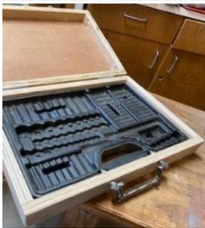
by cutting off the exterior back of the box and reinserted it into the new box. The upper part of the box will be fitted to hold the various tools shown in the photo. It was simple to make with "Wink Wood". Outer frame is 3/4" plywood and the top and bottom panels are 1/4" plywood. Frame assembly was with a Kreg jig, screws and glue. The finish will be light gray. —**Mike Turner**.
