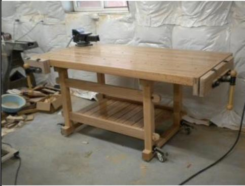
Is a workbench ever finished? I added a lower shelf to mine, of the same Water Oak, 3/4" thick slats, resting on and screwed to cleats on the ends. Like the rest of the bench, 4 coats of urethane. I still have to make an easily removeable attachment for the metal vise in the left rear.
