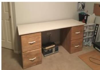
A fun first time project for **Mark Womack** was a desk that his wife pretended to like to two years. So Mark came up with a new design using Sketchup. Joinery is pocket holes and glue. Handles from Hobby Lobby. Mark finished with water borne polyurethane because oil based yellows over time which Mark didn’t want.
