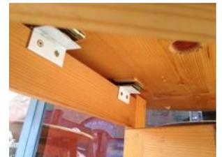
The design for this folding table came from tables at a sidewalk café that **Mike Hardy** saw while in Innsbruck, Austria, a few years ago. Mike made the table of clear pine with a shellac finish. The third photo is of the original table showing how to allow the top to fold down.
