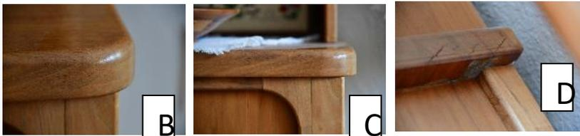
My other little mistake came when joining the top to the base. The sides of the base cabinet are walnut plywood, glued into grooves cut into the corner posts and the top. I cut the grooves using a newly acquired router (non plunge), and it got
