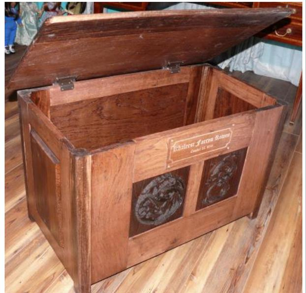
**Gary Rowen** crafted this toy box for his great granddaughter. It is made of hickory, red maple, and some plywood. Gary used a CNC router to carve the 3D panels. The box is stained in red mahogany and coated with urethane. Torsion hinges prevent the lid from slamming closed onto the latch-free box.
