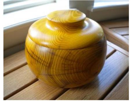
I made this pumpkin lidded bowl out of Osage Orange, with super glue to fill all the cracks. I added some grooves on the bottom, and contoured the lid to fit neatly. I also sanded it to 2000 grit. There is nothing on the wood; it is so hard, you can polish the surface smooth and shiny. 9" diameter, 6" tall with lid.
