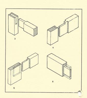
Tenons that meet in a corner must use the maximum possible gluing area to be strong.
