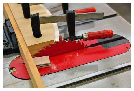
The rail was clamped to the jig, one end of the jig set against the stop block, and the first end trimmed.
