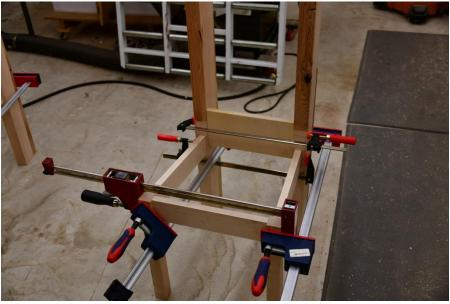
With the chair still clamped up, the exact size of the back rail can be measured.
