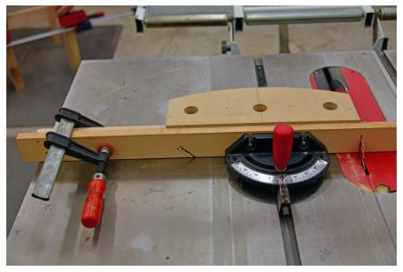
I built another jig to hold the curved rails for cutting to final size and for drilling the dowel holes.
