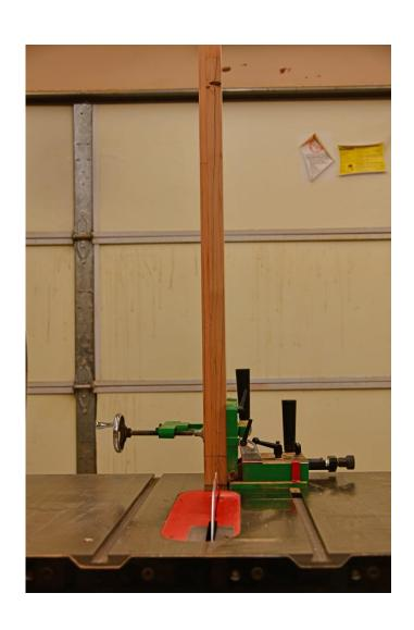
The second cut was made with the leg mounted vertically in a tenoning jig
