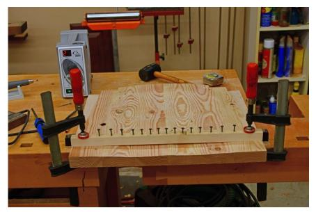
The first method worked, but seemed a little crude (and slow), so I built a jig that allowed for more accurate transfer of the seat contours
