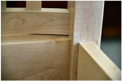
I added a curved reinforcement that is glued to the chair back and the back chair rail
