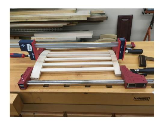
With the dowelling done, the back could be fitted together to test how it looked
