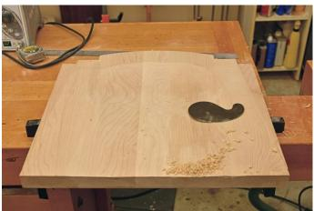
Then smooth the contours with a rotary carver and a spherical burr, followed by random orbit sander until carving marks are gone, then final scraping to even out a few bumps
