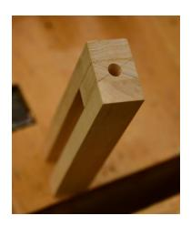
I made a jig for dowelling the slats using offcuts from the slats themselves
