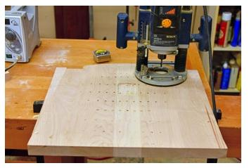
Drill a matrix of holes to mark the depth contours and rout out most of the waste
