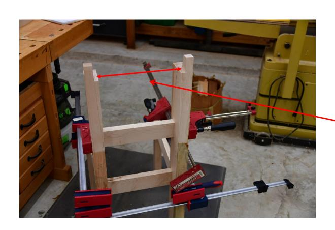
Here's the chair, clamped back together, with the reference surfaces cut on the back legs
