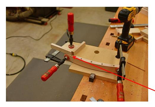
The holes in the slats were drilled along the axis of the slat. This meant that the holes into the rails themselves had to be drilled at the correct compound angle.
