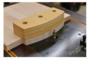
Seat blanks are trimmed to final width, front is cut square and notches are cut. Start on the curved section by marking the position using the plywood template.
