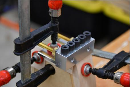
To drill the dowel holes in the top rail, I used the regular dowelling jig, with a second jig to position it correctly with respect to the rail.
