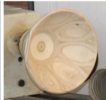
Showing slides of how he prepared and assembled eight pieces cut using compound angles to form the sides of a bowl (as opposed to using a big chunk of wood from a log), **Lon Kelley** was able to turn these neat bowls. The cutting board was made from Wink wood – a very interesting pattern. Lon finished with Minwax natural and wax.
