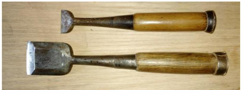
At the top is what used to be an excellent chisel, but is now just, to be polite, a nub; the lower one is a still usable example for comparison. Why was this chisel still in the tool roll? It's too short to sharpen. It's too short for self-defense. In a stretch, one might use it as a scraper but there were six of them. Conclusion: the old carpenter couldn't bear to throw it out. Worse: why do I still have the nub? Conclusion #2: I need a twelve step program for tool addicts.
