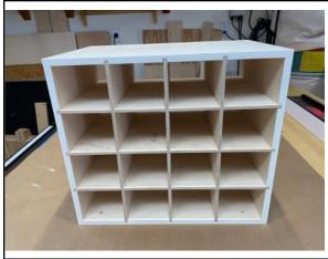
Made an organizer for my daughter's pantry to hold Ziploc storage bags, etc. Constructed of 1/2" and 1/4" Baltic birch, with the inserts joined by a wine-box style mechanical joint. Four screws in the bottom attach the organizer to the shelf. — **Sonny Lawson**
