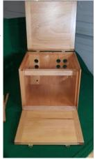
egraph transmitter. He had plans drawn up by another ham radio operator. Made from Alder salvaged from the infamous dumpster. I used a little natural Minwax stain and two coats of spray semi gloss polyurethane. The real challenge was finding slotted brass screws, as Phillips head screws were not widely used at the start of World War II. Apparently they had been invented in the late thirties — **Andy Tofuri**
