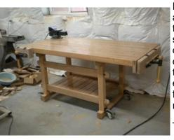
Is a workbench ever finished? I added a lower shelf to mine, of the same Water Oak, 3/4" thick slats, resting on and screwed to cleats on the ends. Like the rest of the bench, 4 coats of ure-thane. I still have to make an easily removeable attachment for the metal vise in the left rear.
