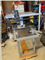
It is a mobile base for a 10" Dewalt table saw. The base is designed to fold up the legs and then roll the saw to transport it or use it at the jobsite. The base is made of 1 1/4" steel square tubing, 1/16" wall. The length of the base frame is 36" and has a width of 16". The legs are designed to fold up underneath in order to transport. Once you
