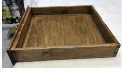
Burak. I used mortise and tenon joinery for the base and wood buttons for the top. The drawer is dovetailed with drawer slips. The finish is aniline dye with Watco Danish oil and General Finishes Arm R Seal.
