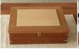
**Mike Hardy**: Pictures of a jewelry box I just completed. 12" x 10" x 3.5". It is cherry and maple, with a milk painted bottom to the maple sliding tray. The design is adapted from a design in Doug Stowe's "Basic Box Making". Finished with shellac on the inside and Liberon on the outside.
