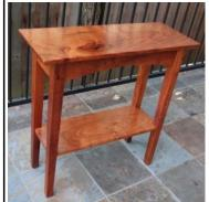
Charles Volek: wall table I recently finished. It is made of Mesquite using traditional mortise tenon joints. Although the shelf appears to cut deep into the penetrates leas.
