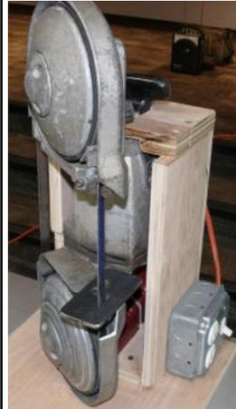
Metal cutting portable bandsaw (Milwaukee portalign band saw) mounted in a cabinet in the vertical position to cut small pieces of metal. It is designed to mount on your workbench with a clamp to secure it or you can remove the tool and use it. There is an electrical switch with a receptacle mounted on the side where you can power up the tool while mounted in the vertical fixed position.
