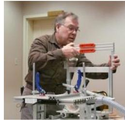
After retiring from his process engineering job, Inventor Matthias Wandell developed a working mortise and tenon machine using the principle of the pantograph to reduce a large scale template to a smaller size desired for a mortise and tenon joint. The machine, using a typical router, takes mortise and tenon making to the next level – a crafter can choose a design for the tenon, or custom make one – a useful tool when designing through tenons where the end of the tenon is exposed.
